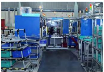
New assembly line with semi-automatic and combined processes ensuring error free product assembly with high productivity. All the processes in this line are closed loop with feedback system and automated dynamic torque checking which ensures the Oil pump's 100% performance.
