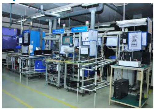
An Electronic Control Unit (ECU) for JCB "Live Link", is a Telematics product assembly line at Plant II. This Telematics ECU line is a state-of-the-art assembly line with Real Time GSM based product assembly and fully automatic inspection carried out through external software. This ensures zero defect during assembly and server based traceability from the field.
