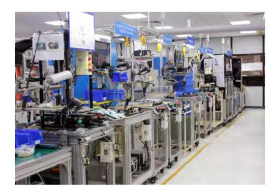
New assembly line with process interlock for Royal Enfield's Driver Information System which conforms to BS IV standards and includes advanced features like LCD Compass.
