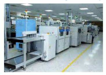
Advanced automated SMD Mounters, Printers & Robotic Machines which are being used to place Surface Mount Devices (SMD) onto Printed Circuit Board (PCB) for Electronic Clusters. They are used for high speed, high precision placing of broad range of electronic components like capacitors, resistors, integrated circuits onto the PCBs.
