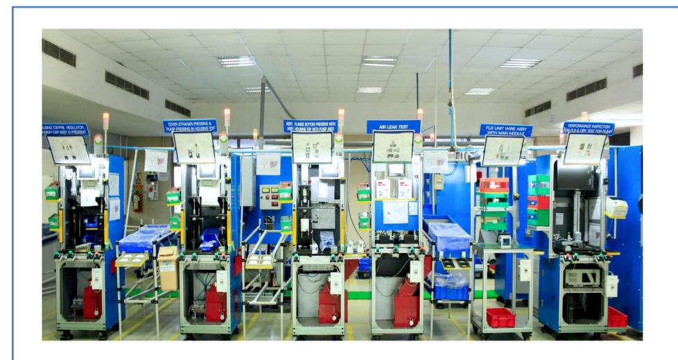
Fuel Pump Module Assembly Line in Plant 2
