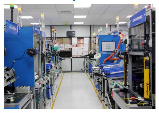
New assembly lines with No Fault Forwarding (NFF) principle ensuring higher quality focus through essential mistake proofing in every step of the process. Barcode traceability in each step of the process, from start to finish of the assembly line.
