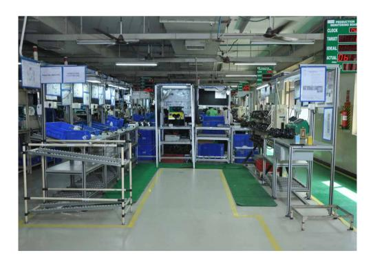
Semi-Automatic assembly line with closed loop processes for assembling Honda Shine Cluster. This assembly line ensures defect free assembly with higher quality control.
