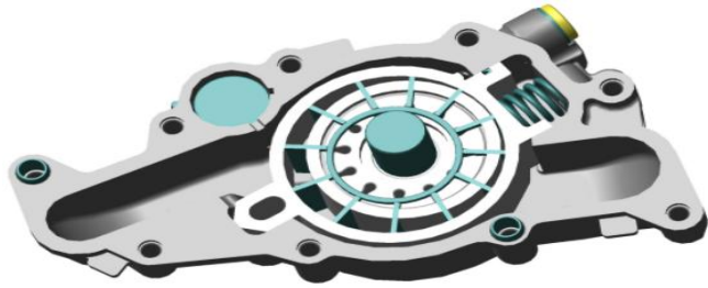
Variable Displacement – Vane Type Oil Pump
